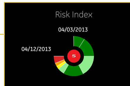
The risk index ring shows the varying risk index stages the transformer has been in over a 9 month period, with the current risk index in the center.
