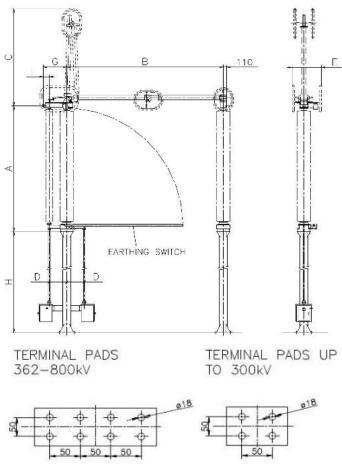
Customised layouts available upon request. Phase-to-phase distance defined by substation layout.
