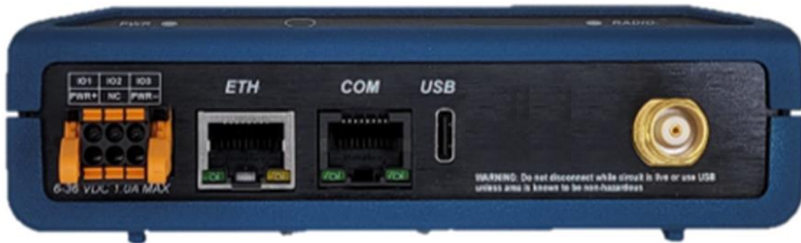
Figure 2-3. TransNEXT, Connectors and Indicators
