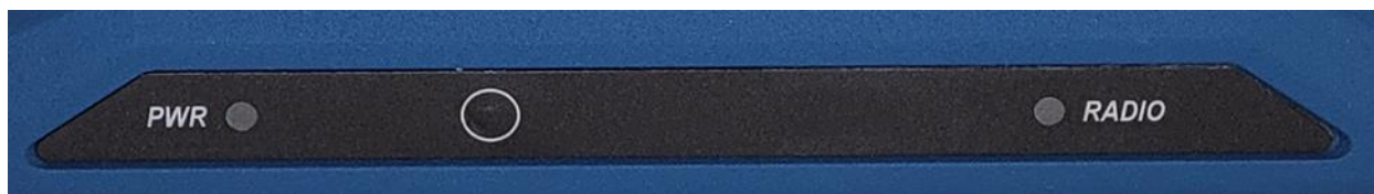
Figure 2-6. LED Indicators & Push Button
