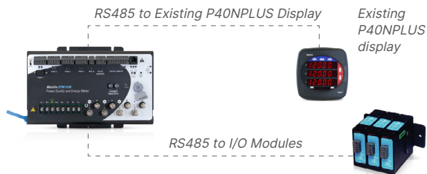
Easy direct retrofit for EPM 9450/9650 utilizing existing I/O and P40NPLUS display
