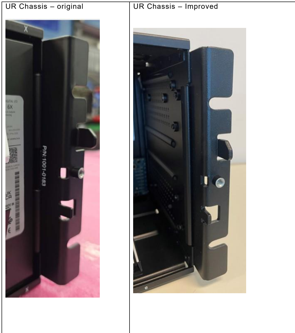
Figure 7 Inside wall of UR chassis
