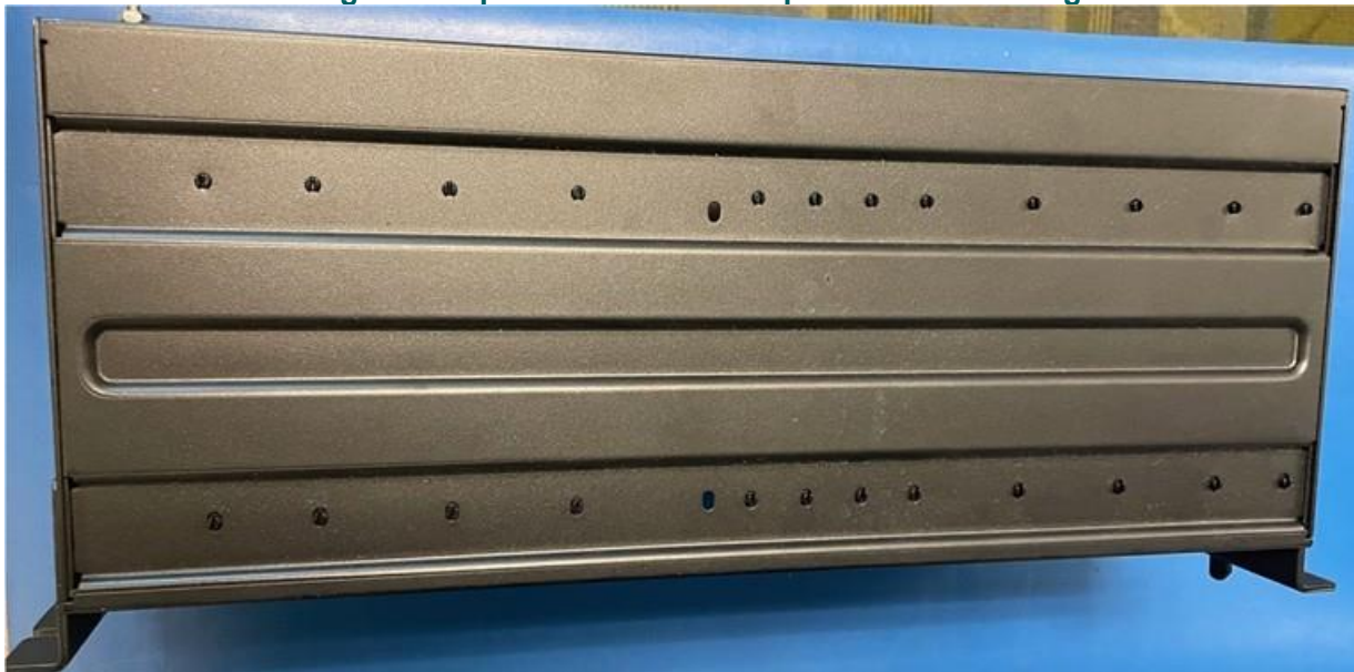
Figure 2 Top of UR chassis – Improved with forming
