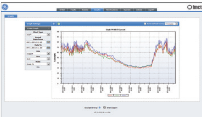
3 phase current profiling identifies magnitude of line imbalance at each measurement point
