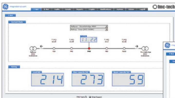
Application displays current line loading and available capacity based on the CIGRE algorithm
