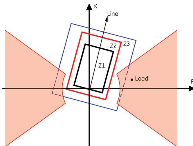
Distance relay quadrilateral characteristics supervised by the load encroachment function.
