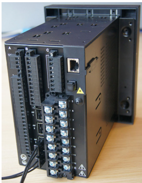
Figure 2-20: AF point sensors connected to 350 relay
