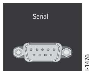
Figure 19: Serial port RS232 and RS422/485
