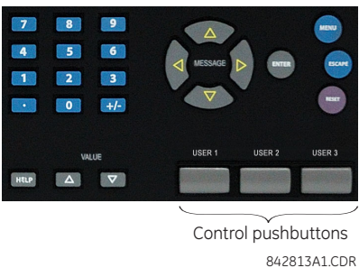
Figure 5-50: Control pushbuttons (enhanced front panel)
