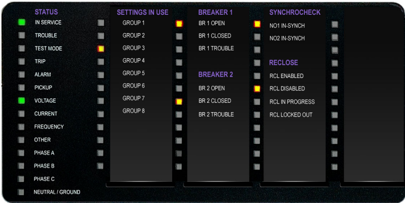
Figure 4-48: Typical LED panel for enhanced front panel
