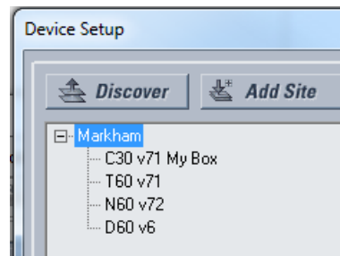
Figure 3-66: Discover button to detect UR devices in network
