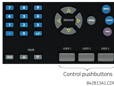
Figure 5-53: Control pushbuttons (enhanced front panel)
