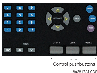
Figure 5-54: Control pushbuttons (enhanced front panel)
