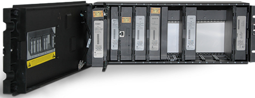
Figure 11-15: Modules inside relay with front cover open (enhanced front panel)
