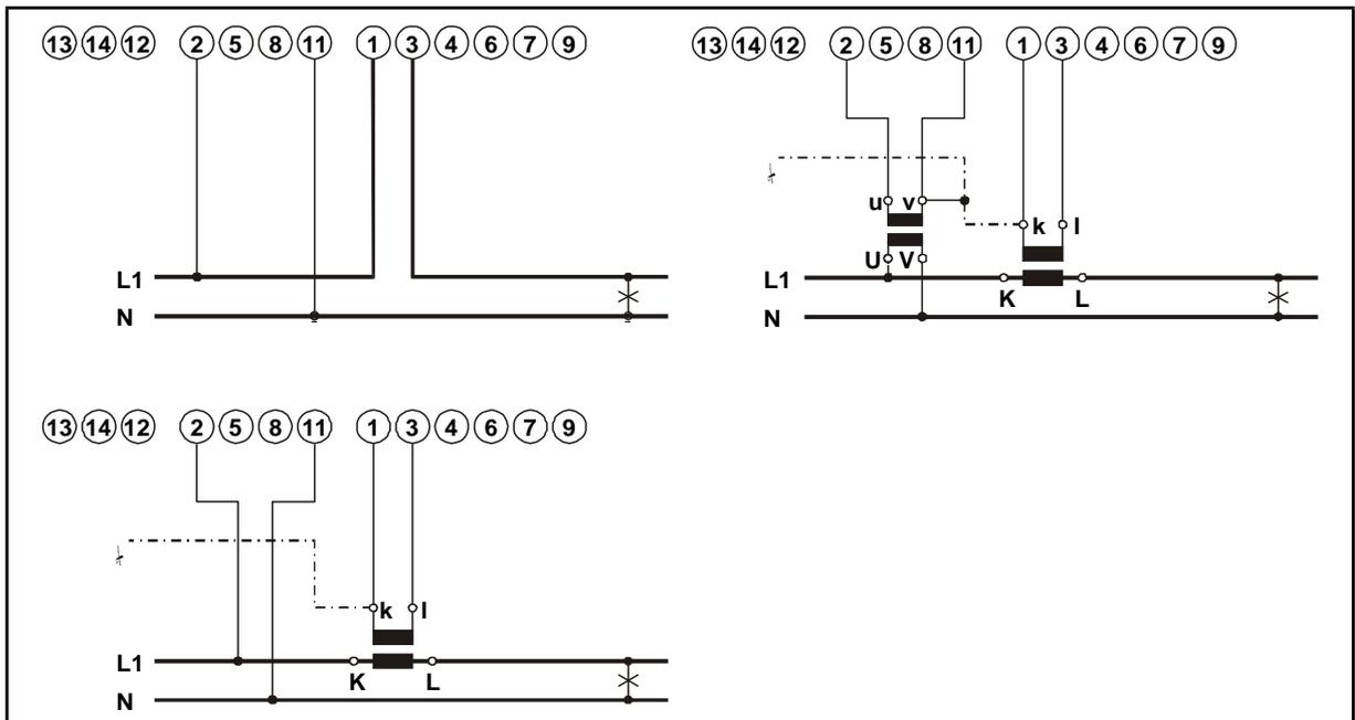
FIGURE 10-2: EXTERNAL WIRING DIAGRAM: SINGLE PHASE (1B)
