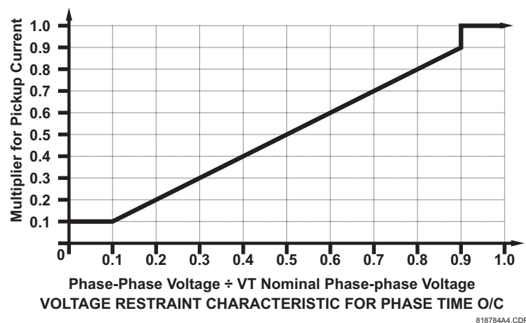
Figure 5-127: Phase time overcurrent voltage restraint characteristic
