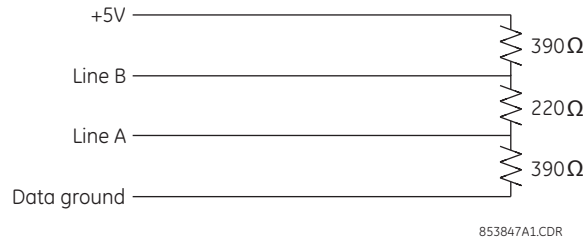
Figure 4-2: Profibus termination
