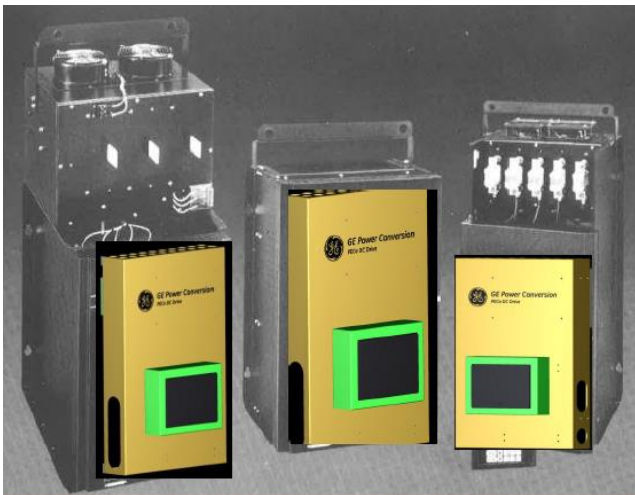
Proposed hinged swing-out controller mounted on the existing power module
