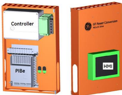
Proposed hinged control door assembly
