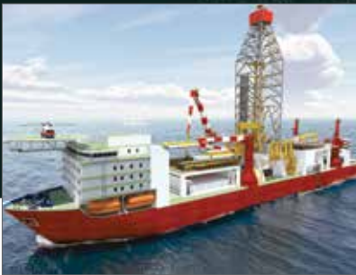
Transocean Deepwater Drillship Integrated vessel and drilling power, e-propulsion and DP
