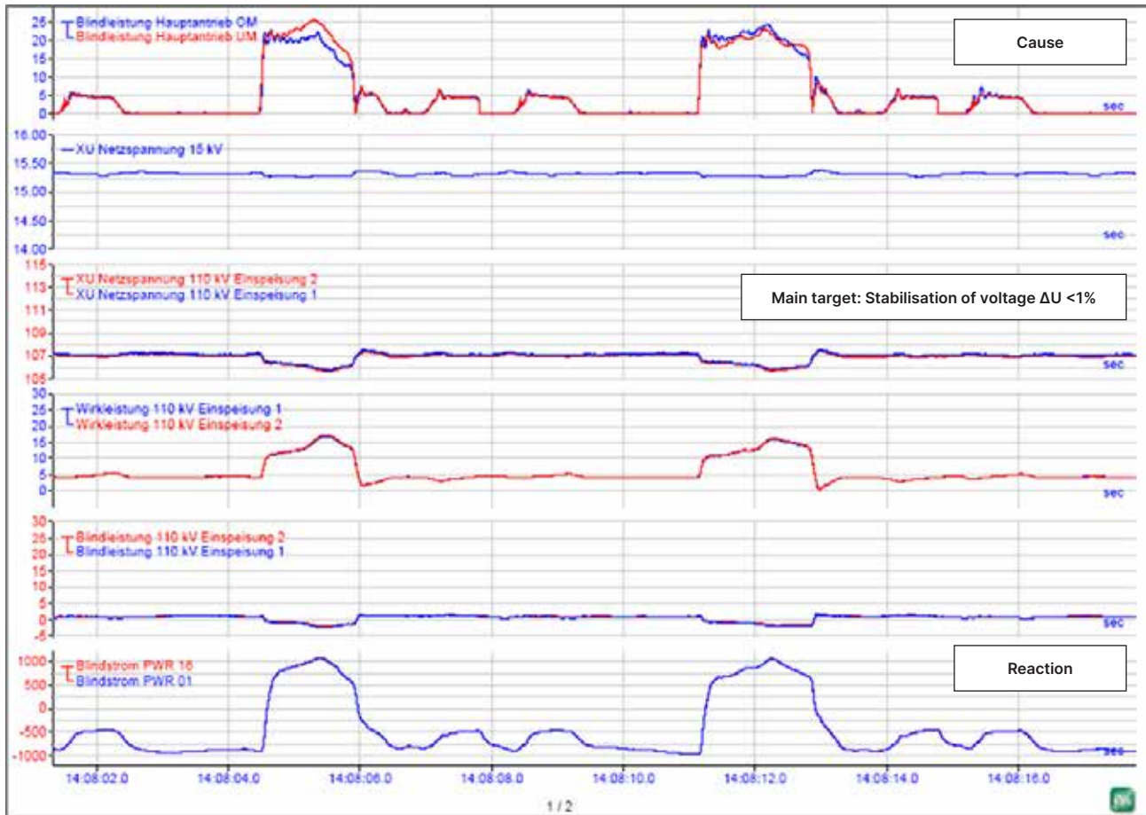
Figure 9: Measured traces (5 ms sampling) of the operation of the dynamic compensation on the rolling passes of the main drive. Curve for 15 kV and 110 kV voltages, real power, reactive power of the 110 kV supply.
