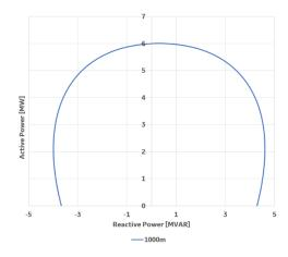
$13. \ Sample \ PQ \ diagram \ for \ \textit{FLEXINVERTER} \ 2090 \ at \ nominal \ grid \ voltage, \ 1400 \ Vdc \ and \ 35^{\circ}C \ ambient \ diagram \ for \ extra \ extra \ for \ extra \ extra \ extra \ for \ extra \ e$
