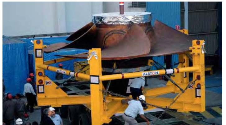
Biggest Kaplan runner ever manufactured in India at the Hydro Vadodara facility
