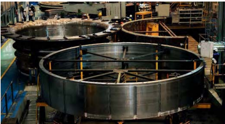
Manufacturing of large hydro project component at Vadodara facility
