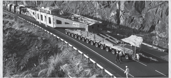
Alstom's 800 kV HVDC transformer enroute from Vadodara to the project site at Champa
