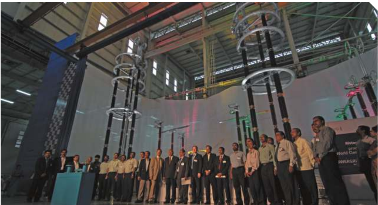
World's first 1200 kV Double Knee Type Disconnector manufactured at Padappai factory for Power Grid's 1200 kV national test station located in Bina
