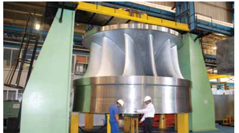
Hydro turbine, Francis Runner balancing in progress, India
