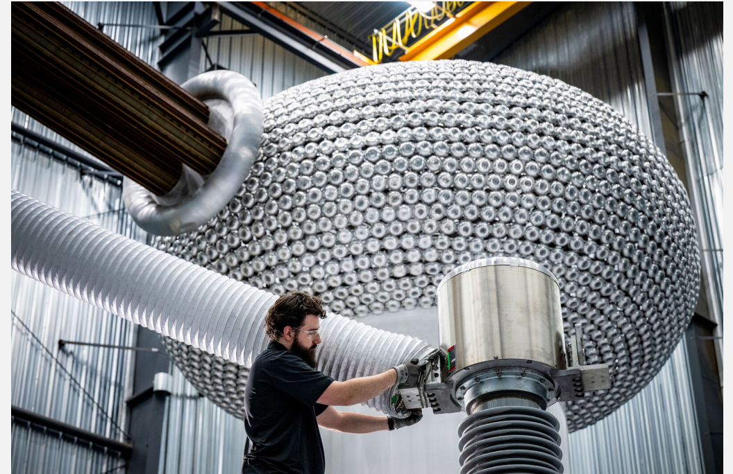
Connecting a transformer to a high-voltage generator in Charleroi, PA.
