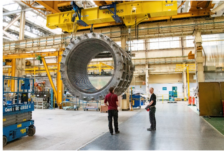
A synchronous condenser under construction in Rugby, UK, where GE Vernova is manufacturing equipment for Transgrid to help stabilize the grid in New South Wales, Australia
