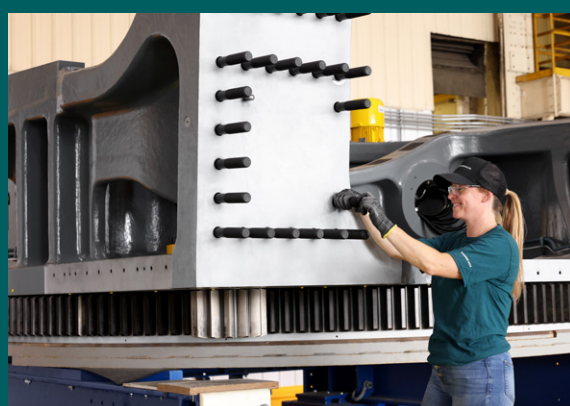
A technician installing hardware on a wind turbine bedplate in Schenectady, New York
