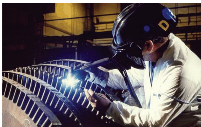
Blade tenon repair
