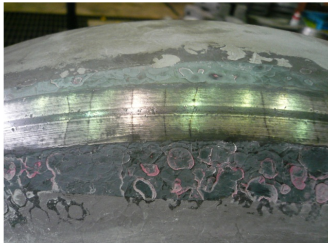
Cracking on the contact surface of a valve head
